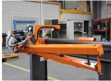
By using a gripper for longitudinal movement, there is no need for a slow and big industrial robot. Furthermore, the material's position is always known.
