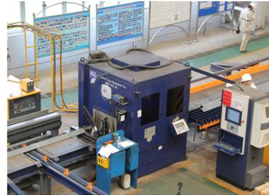
The closed cutting cell includes inside noise absorption material to reduce noise outside the cutting cabin. Furthermore, it has very effective fume extraction.
