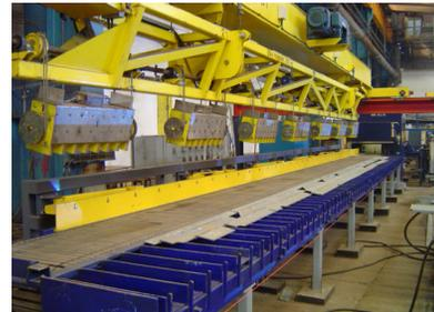
HGG can also provide a magnetic loading crane for efficient loading and unloading of profiles and cut parts.
